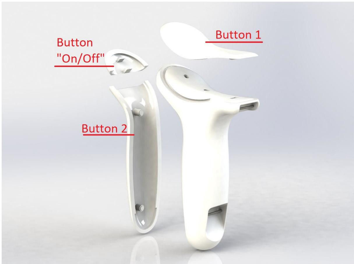
*Pic.4. The way the buttons must be removed for cleaning.*
